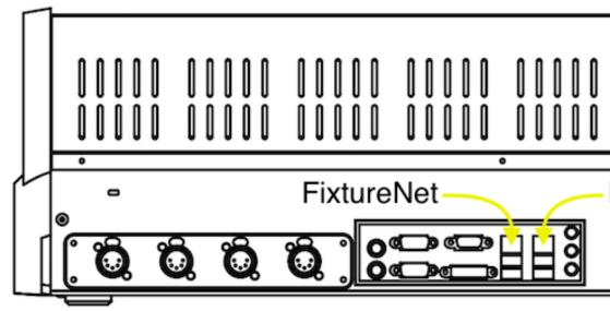
Figure 36.1. Back panel of RoadHog 4 Console
