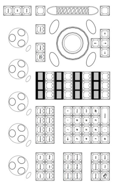
Figure 32.2. Programmer section of the Hog 4 front panel
