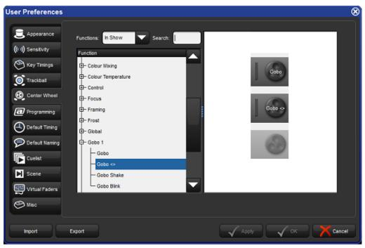
When a fixture selection is made functions assigned to the center wheel will be diplayed on the toolbar located at the bottom of the front panel's center display. Functions that you've assigned to the center wheel wil only be displayed if they are valid for your current fixture selection.
