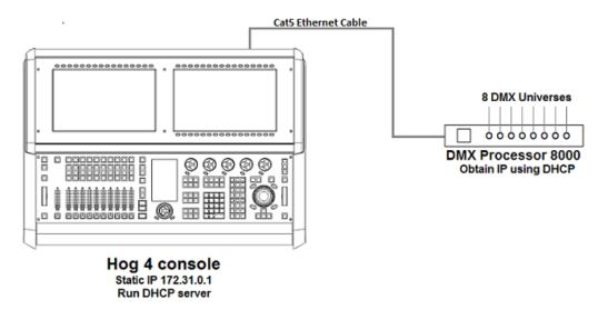
**Example B:** The console is a DHCP server, and all other nodes obtain an IP address from it.
