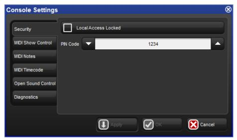
Figure 3.7. Security Settings Tab of Console Settings Window
