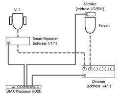
Figure 5.4. Examples of Fixtures requiring Multiple Patch Points
