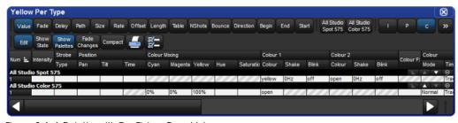
Figure 8.4. A Palette with Per Fixture Type Values
