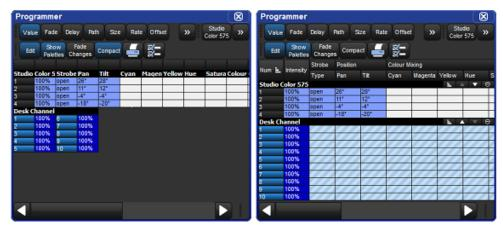
Figure 2.12. A spreadsheet with and without Compact Mode
