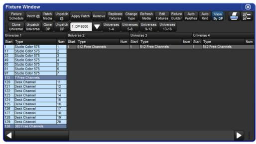
Figure 5.3. The View by DP view of the Fixture window
