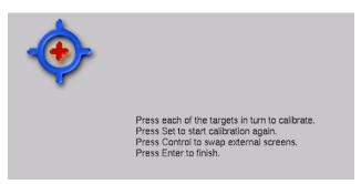
Figure 3.2. The Calibration Screen
