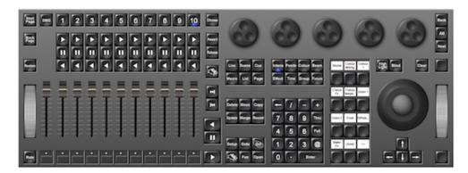
The front panel of Hog 4PC looks and behaves very similarly to the front panel of the Hog 4 console. Click on buttons to simulate pressing keys on the console. You can also click and drag to alter the various encoders or faders. In addition, when you right click on the trackball, it will illuminate blue allowing you to then left click and drag on the trackball to adjust the pan and tilt of the selected fixtures.
